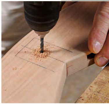
Position the legs and predrill the subtop. After locating the legs (right), Coleman drills a centered clearance hole for a screw into each leg (above).
