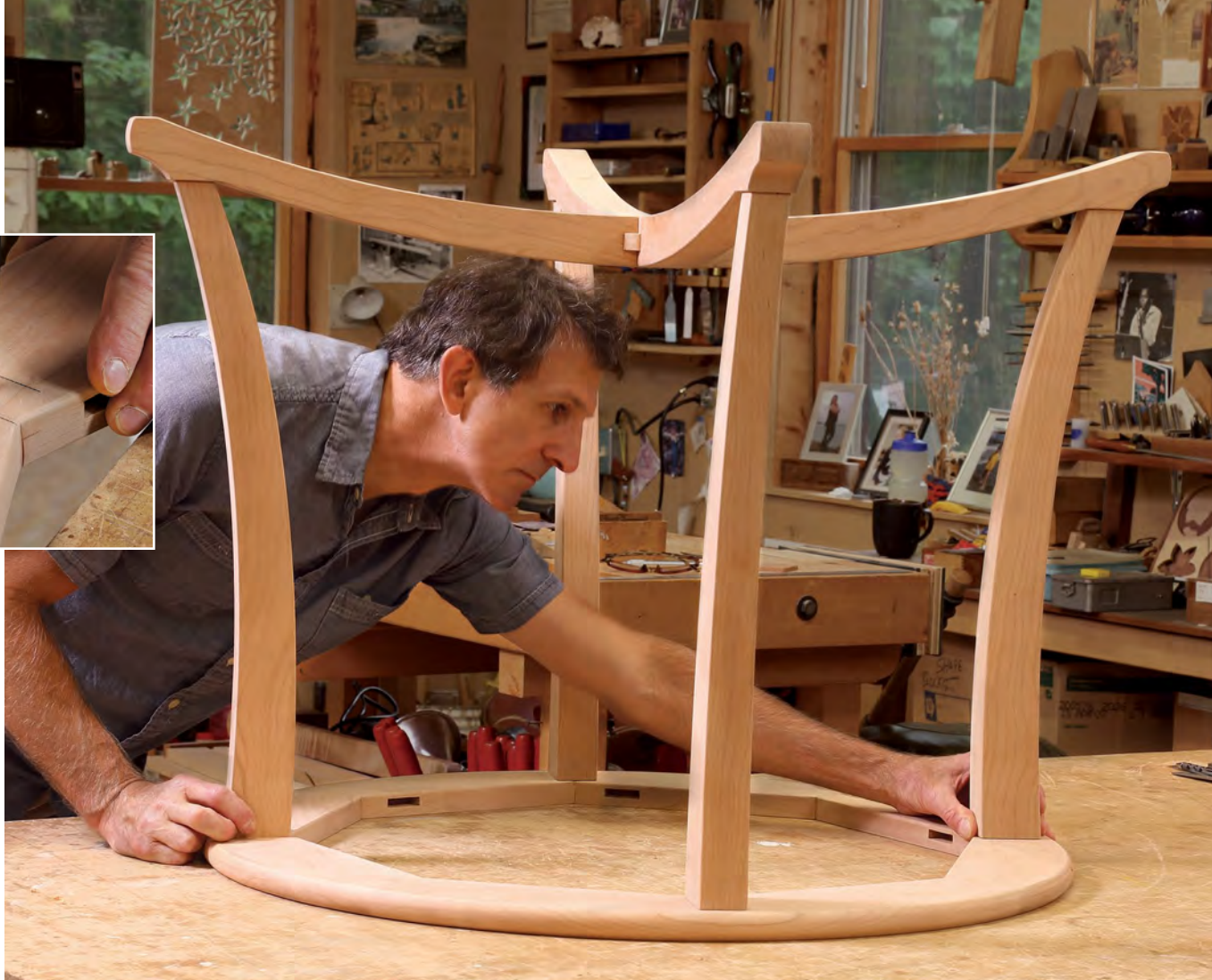
Position the legs and predrill the subtop. After locating the legs (right), Coleman drills a centered clearance hole for a screw into each leg (above).
