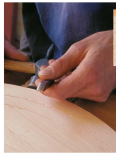
Crescent lays the groundwork. Referring occasionally to his sample pattern, the author begins a pattern by stamping the large crescent, judging the spaces between marks by eye.
