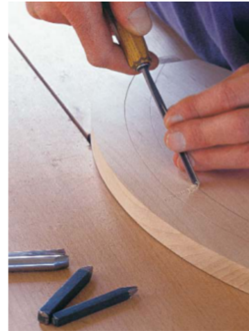
Begin with a V-groove. The author follows a pencil line with a V-parting tool to cut grooves that establish the radius of the pattern.
