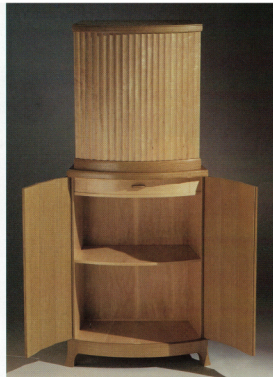
Coved and coopered. Coleman handplaned the solid maple upper door. The white oak lower doors are veneered coopered panels.
