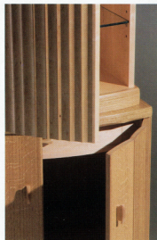
Coved and coopered. Coleman handplaned the solid maple upper door. The white oak lower doors are veneered coopered panels.
