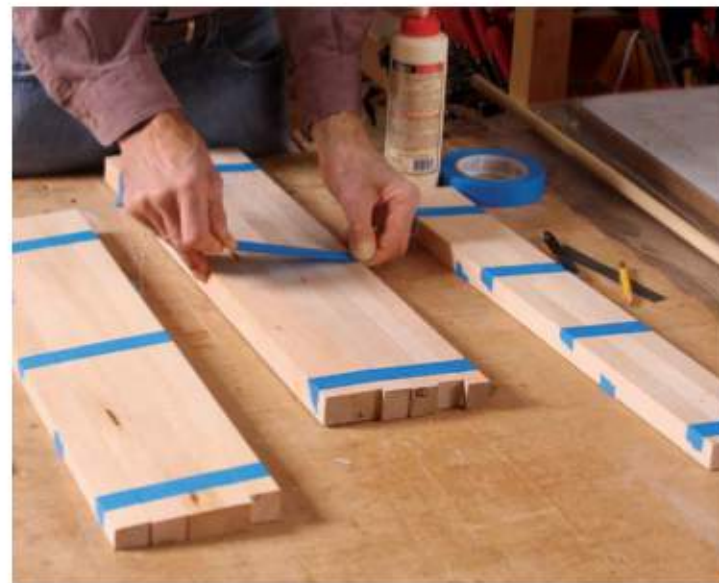
Get an angle on the staves. Set a bevel gauge to closely match the curve along the top of each stave.
