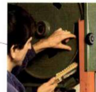
Keep it clean. For best tracking, brush the bandsaw's tires regularly and start a veneer-cutting job with a fresh blade.
