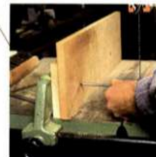
High fence provides full support. The auxiliary fence should be at least as high as the veneer will be wide.
