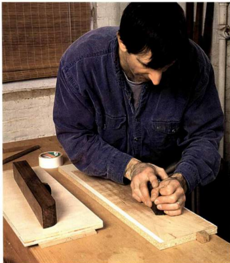
Smoothing after sawing. Double-stick tape keeps a sheet of veneer still for a quick smoothing with handplanes. At \frac{1}{16} in. thick, the veneer can be planed and worked like solid wood.
