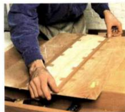
Taping under way. Short pieces of veneer tape are moistened and stretched across the joint; when they dry, they pull the joint tight. A lengthwise strip of tape reinforces the temporary joint.
