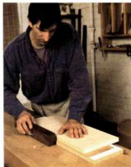
Shoot the edges. A stroke or two with a jointer plane prepares the veneers to be joined edge to edge.
