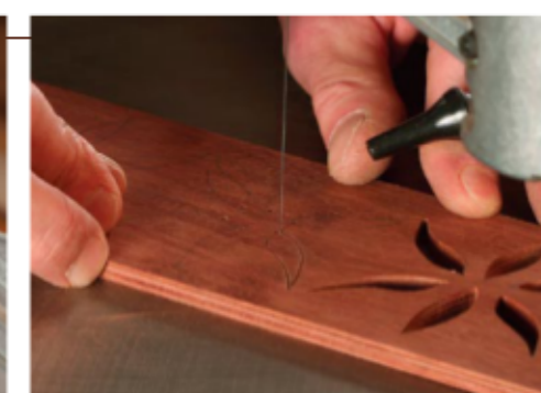
Make the cutouts. Drill holes through the cutout areas to make way for the scrollsaw blade. Cut slowly and carefully on the line. To create a repetitive pattern on multiple pieces, tape the layers of veneer together, and cut them all at once.
