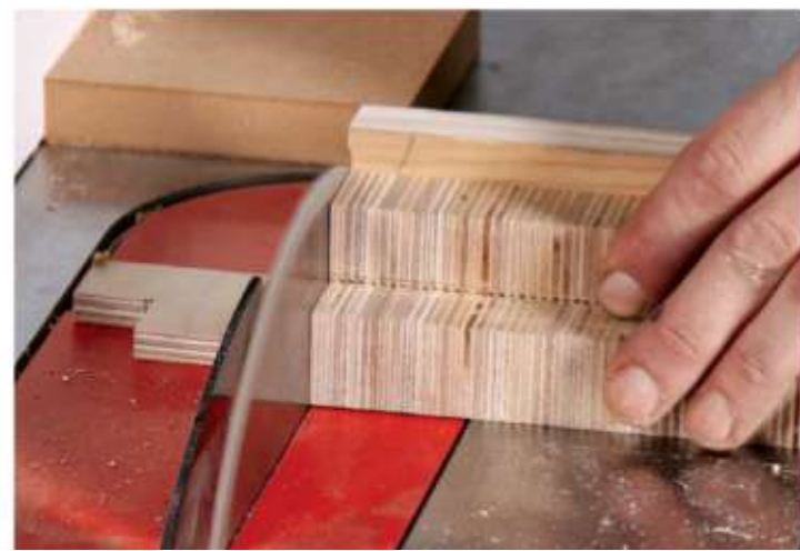
Frame job. Hansuld’s coffee table has 19 mitered frames, each one reinforced with plywood L-tenons.
