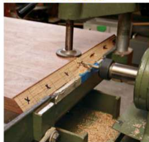
Cut the joint. Coleman cuts his miters first, then cuts the mortises with a horizontal mortiser. A router or Domino would work as well.
