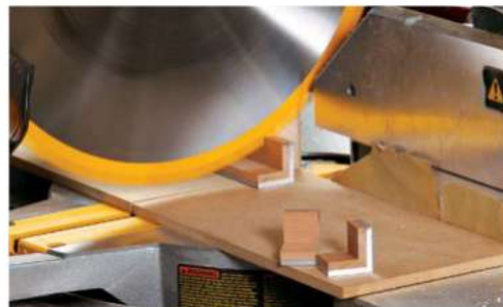
Chop chop. A regular woodworking blade in the chopsaw (or tablesaw) makes quick work of cutting the long blank into dozens of tenons.
