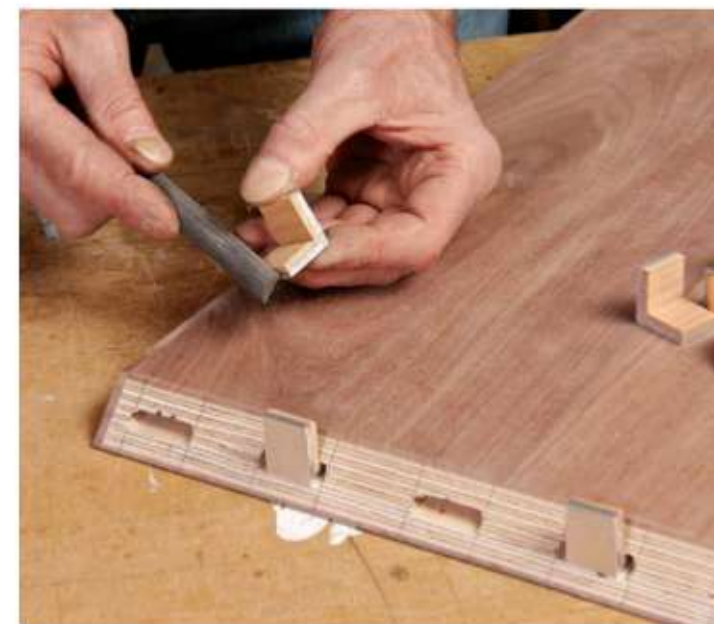
Chamfer if you must. A few strokes with a file ease the edges of the tenons. To avoid having to round over the side edges of the tenon, Coleman makes the mortises extra wide.
