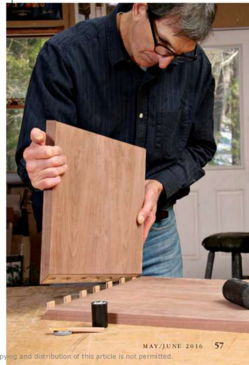
Two-step glue-up. Coleman glues his tenons into one side of the case and lets them dry, then glues them into the second side. This means that to close the joint he needs clamping pressure in only one direction.
