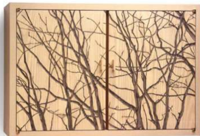
Flowing frame. With the powerful tenons hidden, Gowdy's mitered case works as a clean, elegant border for his carved doors.
