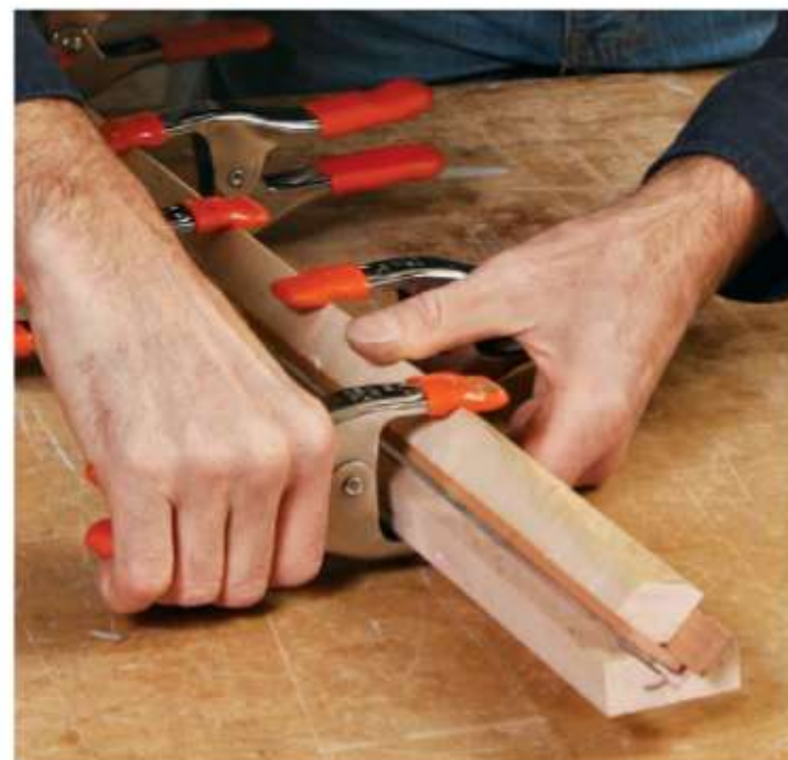
Clamp the sandwich. With the aluminum angle resting in a cradle and the wood strips glued, Coleman uses a square-section caul to distribute clamping pressure. The caul and the cradle are both waxed to resist glue.
