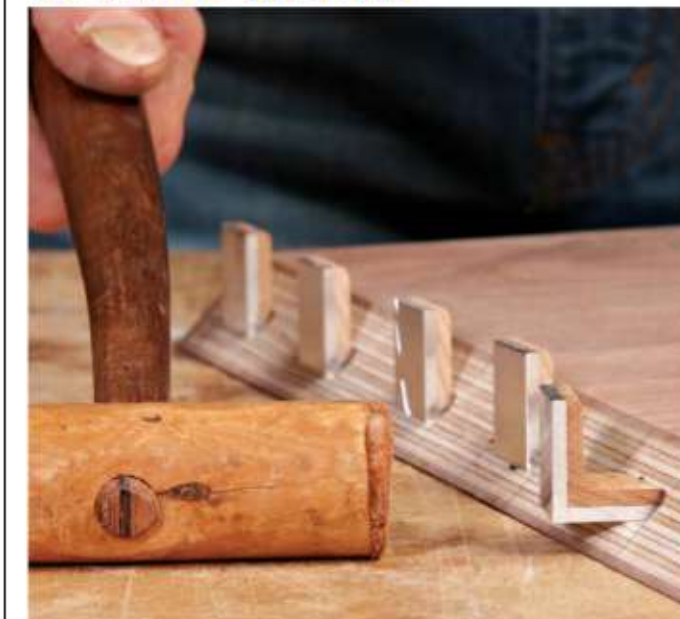
Two-step glue-up. Coleman glues his tenons into one side of the case and lets them dry, then glues them into the second side. This means that to close the joint he needs clamping pressure in only one direction.
