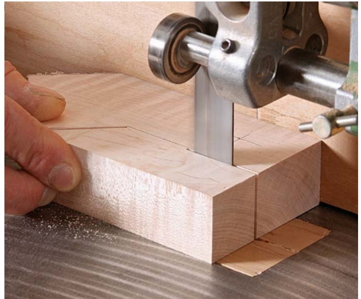
Cut the body to shape. All the cuts are easily made on the bandsaw. Make the angled cuts first (above), then use a fence to finish the straight inside cut (right).
