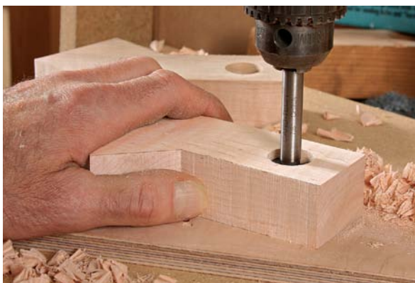
Drill for the post. The post anchors the puppy in the benchdog hole. Transfer its location from the plan and then drill the hole for it using a Forstner bit.
