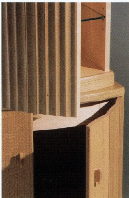
Coved and cooped. Coleman handplaned the solid maple upper door. The white oak lower doors are veneered cooped panels.
