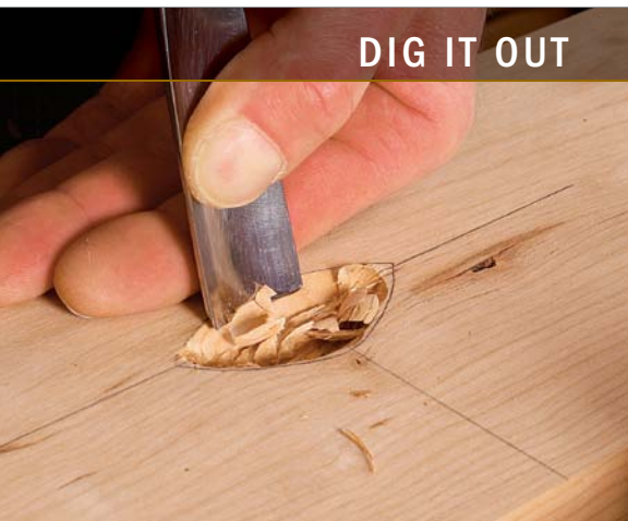
Work around the rim. Use a #8-20mm and #7-27mm gouge to rough in the perimeter. Work across the grain first (left), then with it (above).
