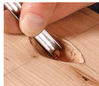
Get under. You need a smaller gouge to create the undercut at the top of the pull (left). Coleman uses a #8-4mm gouge there. In the middle (right), he uses a #8-10mm and a #5-10mm.
