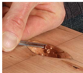
Get under. You need a smaller gouge to create the undercut at the top of the pull (left). Coleman uses a #8-4mm gouge there. In the middle (right), he uses a #8-10mm and a #5-10mm.
