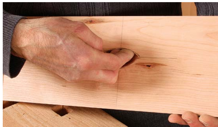
Get a feel for it. Gauge your progress by feeling the pull. You want to be able to grab the undercut comfortably with two fingers.
