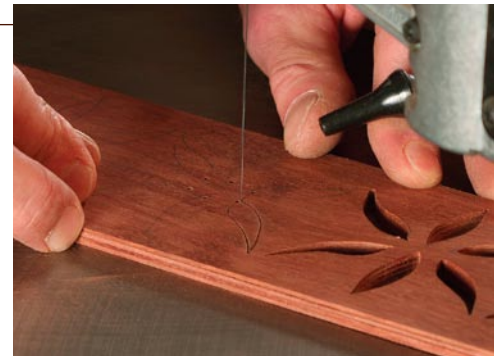
Make the cutouts. Drill holes through the cutout areas to make way for the scrollsaw blade. Cut slowly and carefully on the line. To create a repetitive pattern on multiple pieces, tape the layers of veneer together, and cut them all at once.
