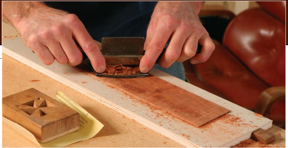
Veneers should be just over \frac{1}{16} in. thick. Resaw both the underlayer and pattern veneers (left). Clean up the material with a cabinet scraper and sandpaper, holding each piece in place with double-stick tape (above).
