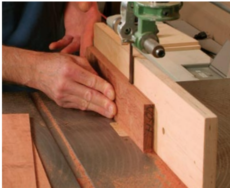
Veneers should be just over \frac{1}{16} in. thick. Resaw both the underlayer and pattern veneers (left). Clean up the material with a cabinet scraper and sandpaper, holding each piece in place with double-stick tape (above).
